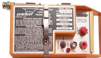
Pointer ELT Similar to that on some ACGP Scouts- (Pointer Electronics)
